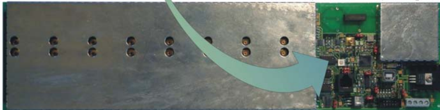
The 8 Channel (Eureka Mux8) or 4 Channel (Eureka Mux4) Multiplexer
