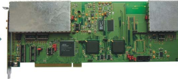
The Eureka PCUF Ultrasonic Flaw Detector Plug & Play PCI Board
