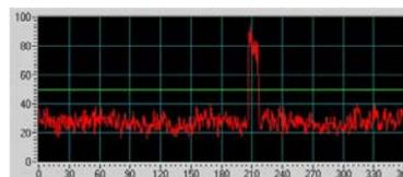
The chart below shows the result of applying the algorithm to the first chart above. It shows both the low and high frequency components being removed and a threshold of 52.4% calculated.
