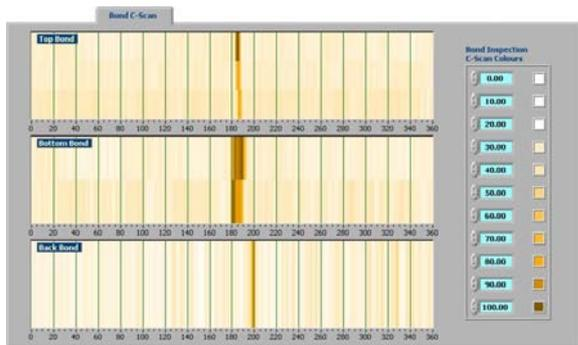
Each line in the C-Scan image is a different channel; therefore in the above case there are 3 channels assigned to the Top bond inspection, 2 channels for the Bottom bond inspection and a single channel for the Back bond inspection.
