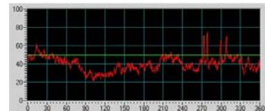
And a high frequency component, which results in the signal randomly, fluctuating. The chart below illustrates this high frequency fluctuation, on a typical piston.
