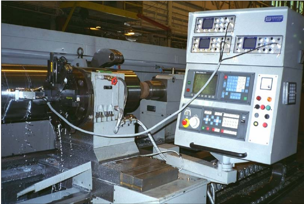
Figure 4 - The Ultrasonic System Inspecting a Roll
