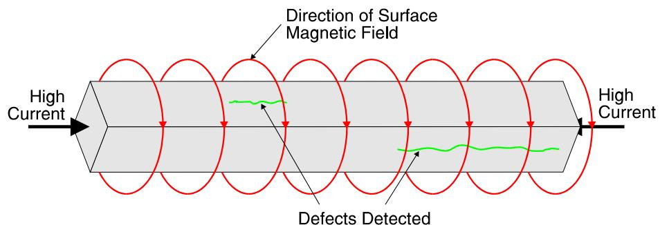
These magnetic particles will migrate through the liquid to the attractive magnetic fields (North and South) produced at the edges of any surface breaking cracks where the magnetic flux leaks into the air.
