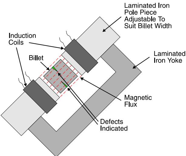
Each yoke magnetises two opposite faces by generating AC flux between the pole piece ends. AC flux with its attendant skin effect will traverse the two opposite sides creating a transverse magnetic field in the required direction. Indicating fluid applied immediately before each yoke will allow particles to move through the fluid layer to the defect edges during the magnetising phase.
