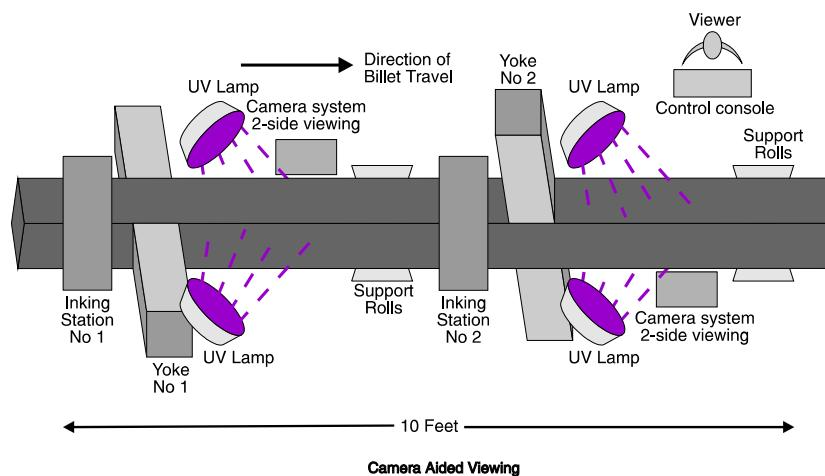
A much more simple and reliable viewing system is the use of low light level, spectrum filtered CCTV cameras, one for each surface with outputs to a single four-way split screen monitor to be viewed in an operator's booth. The operator would be provided with a remote operated marking device to mark defects appropriately.
