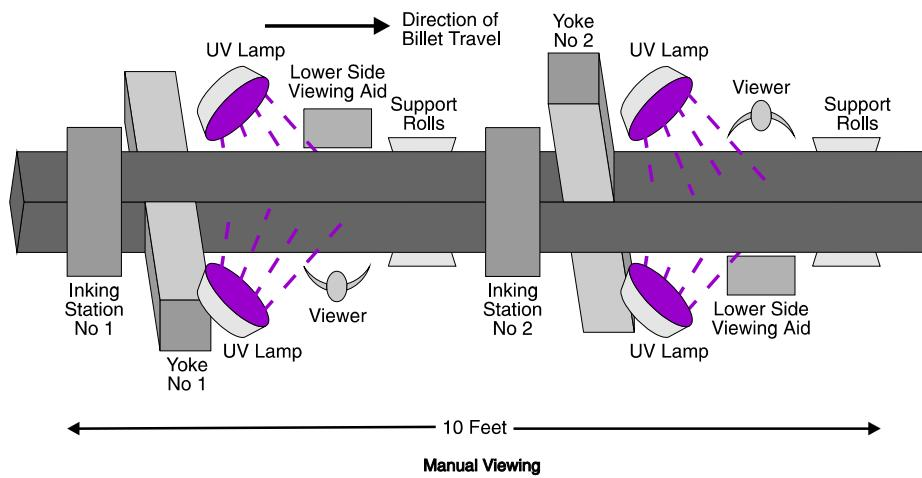
Immediately after each magnetising position is a viewing station. The viewing can take either of two forms. Each of the two viewing stations can have a man to view the upper surface and, with the aid of a specially designed mirror system, the lower surface.
